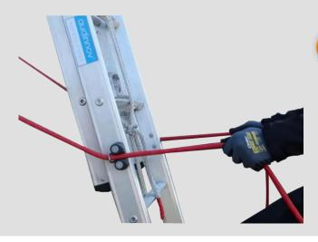
Pull both ends of the rope to put moderate tension.
